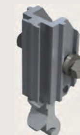
50187-31 Lift-A-Deck II Low Profile Foot Assembly. Machined guide shoe allows for inspection of both locking lugs while beam remains installed in the track. Features a coil spring for optimum service life. Weight: 0.6 lbs./0.27 kg.
